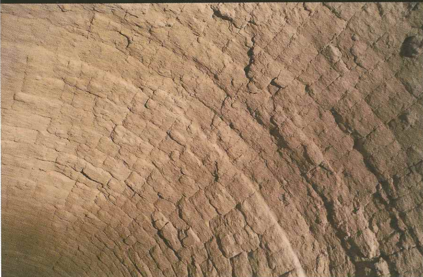
Figure 7: brick surface appearance after use in the transition zone of kiln B
