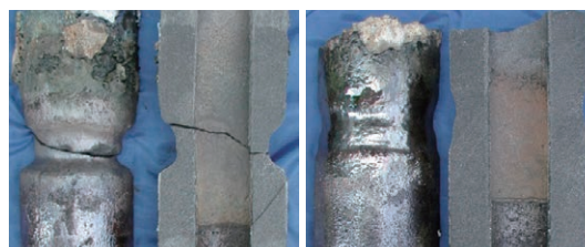
Conventional High Viscosity PRIOS Comparison of SEN Erosion
