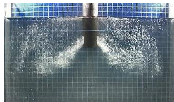
Water model simulation of molten steel flow in the mold
