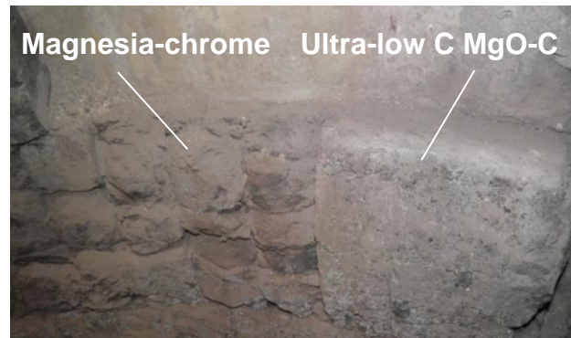
Slag line of steel ladle after use.
