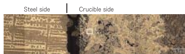
Fig. 4 Microstructure of steel and crucible near interface (Area A in Fig.3).
