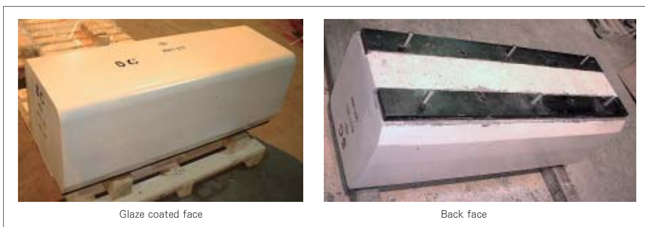
Fig. 2 Appearance of glaze coated block with anchors.
