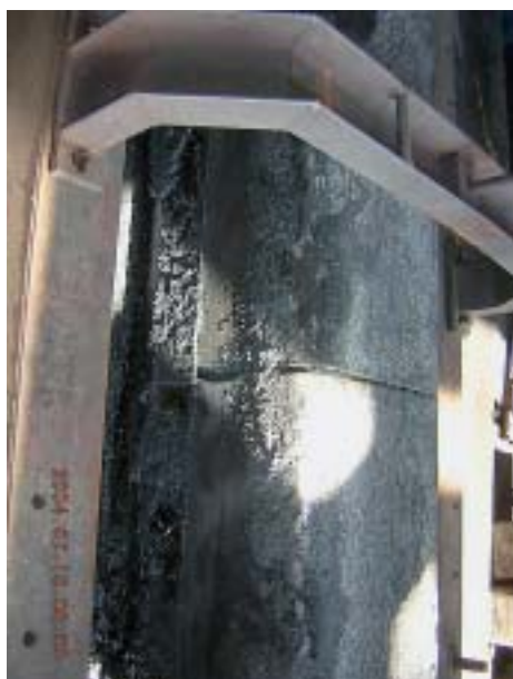
Fig. 3 Appearance of glaze coated block with anchors after 5 months use.
