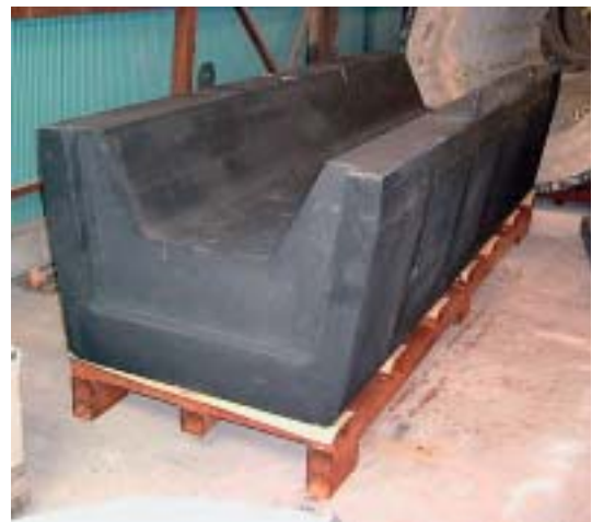
Fig. 5 Large precast block for slag runner.
