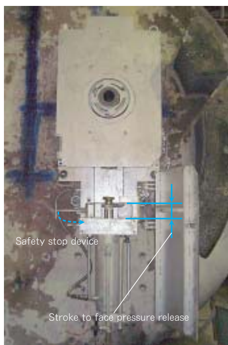
Fig. 2 Photograph of newly developed SV equipment "SST".
