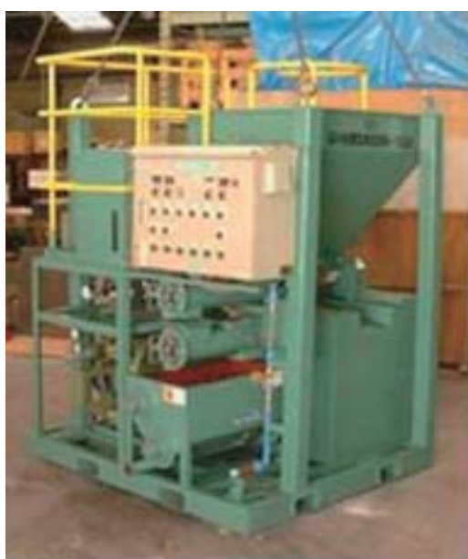
Fig. 2 Low capacity CLS installation equipment.
