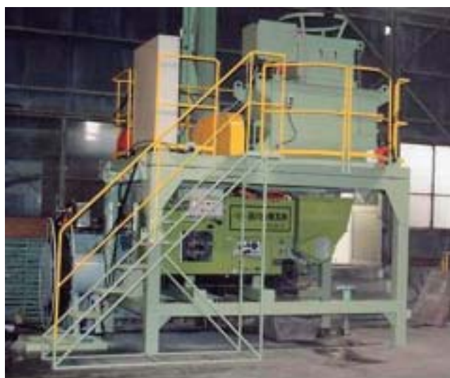
Fig. 1 High capacity CLS installation equipment.
