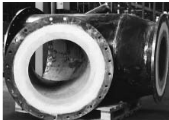
Fig. 3 Representative one body with iron shell products. These are used as exhaust gas ducts.
