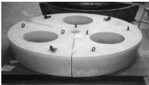
Fig. 4 Large blocks having metal fittings for lifting by crane. Ceiling block of electric arc furnace is typical product.
