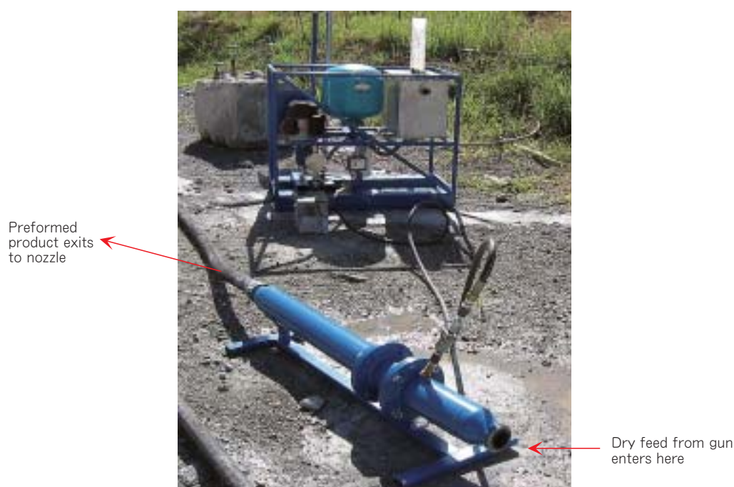
Fig. 3 Inline Preform Mixer attached to Pump Unit.
