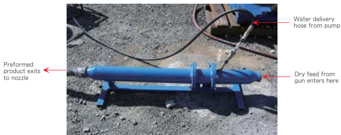
Fig. 2 Inline Preform Mixer Unit.
