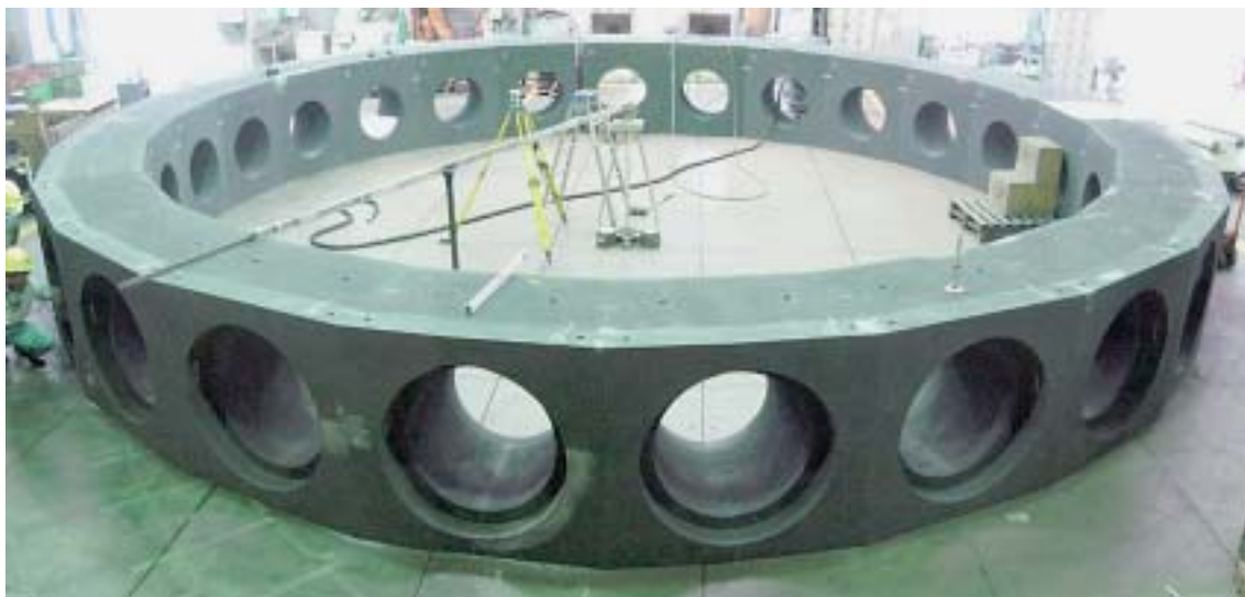
Fig. 8 Trial assembly of newly developed large blocks for blast furnace tuyere.
