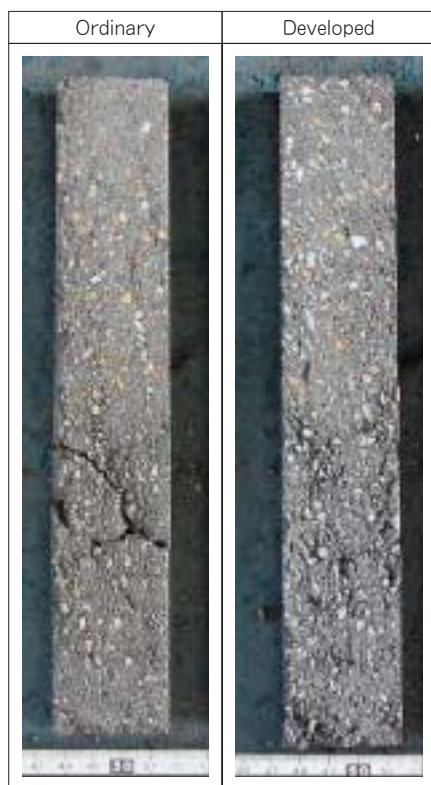
Fig. 9 Cross section of MgO-C bricks for RH degasser vessel after spalling test.
