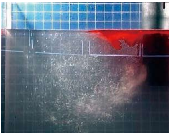
Fig. 3 Entrapment of liquid paraffin (mold powder) by vortex in water model.
