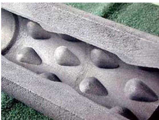
Fig. 9 Inside bore appearance of Mogul SEN.
