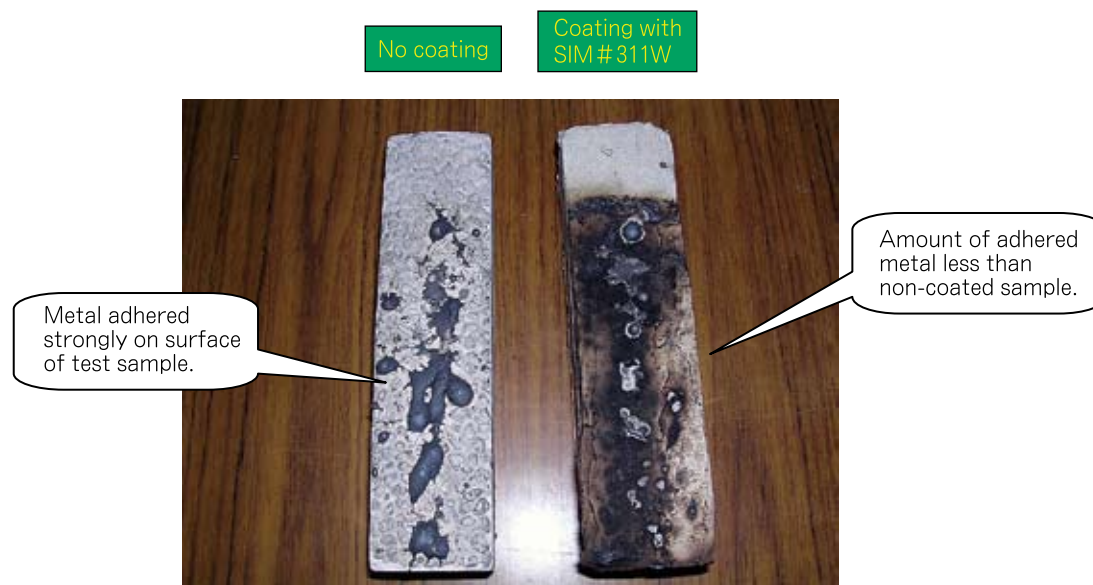
Fig. 5 Samples of insulating unshaped refractory after hot metal dropping test.
