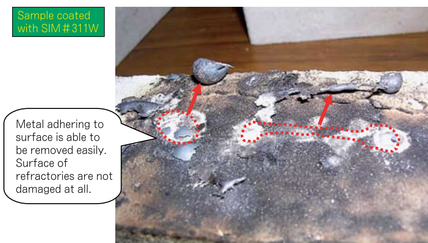
Fig. 6 Prevention effect of SIM#311W on adhesion of hot metal.
