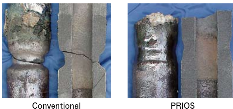
Fig. 7 Appearance of SEN after casting.
