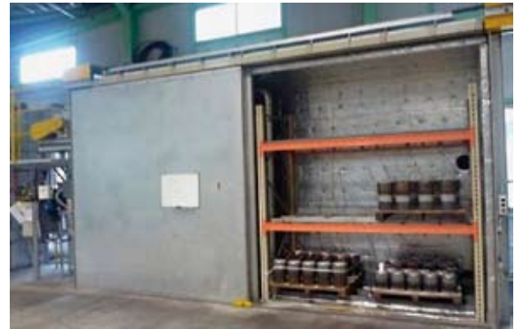
Fig. 3 New dryer for drying steel casing mortar of nozzles.
