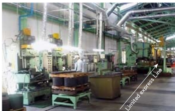
Fig. 6 Express processing line for small lot production.
