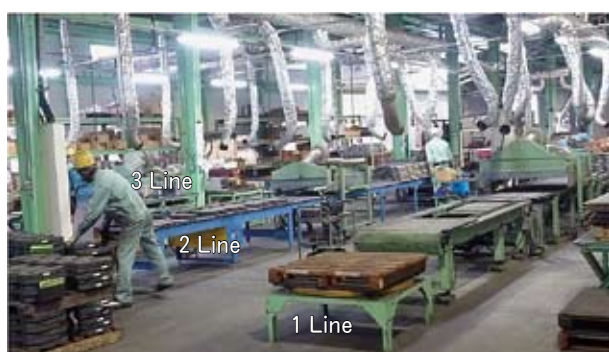
Fig. 5 View of three (3) SV plate furnishing lines.
