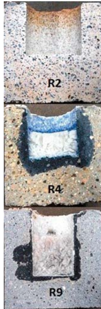
Fig. 3 Results of alkali cup testing at 1100°C with Sodium Sulphate reagent.
