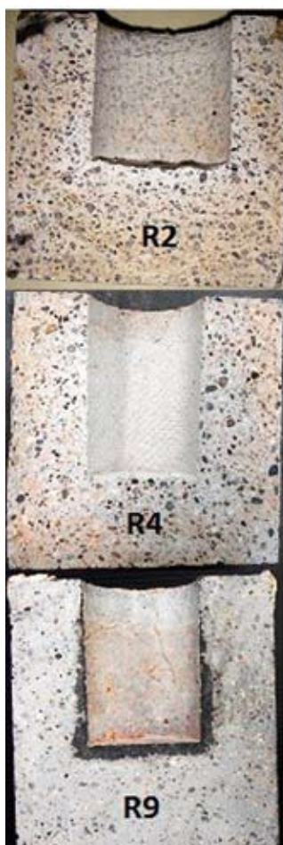
Fig. 1 Results of alkali cup testing at 1100°C with Potassium Sulphate reagent.
