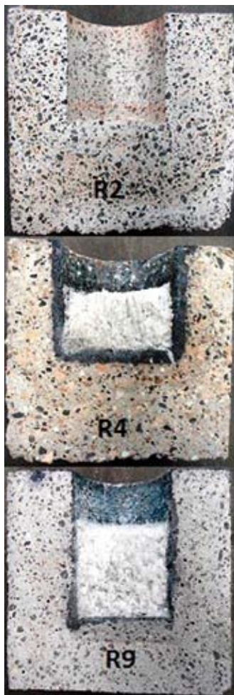
Fig. 2 Results of alkali cup testing at 950°C with Sodium Sulphate reagent.
