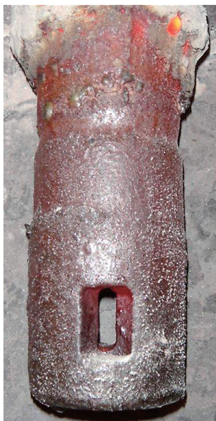
Fig. 7 Appearance of “Bend port” SEN after use.
