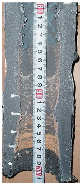
Fig. 12 Cut section of “Mogul with reverse-taper port” SEN.
