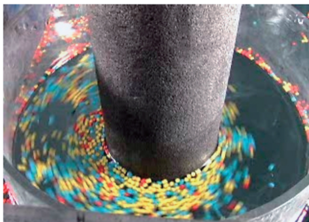
Fig. 2 Swirling flow generated by “Bend port” SEN.
