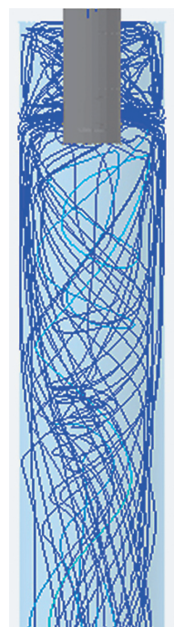
Fig. 6 CFD-calculated streamline for “Bend port” SEN.
