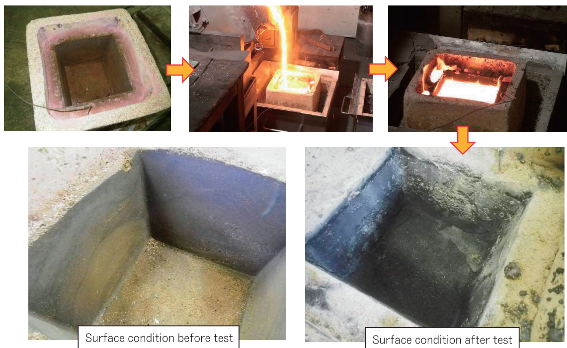
Fig. 3 Procedure of thermal shock test and surface condition before and after test.
