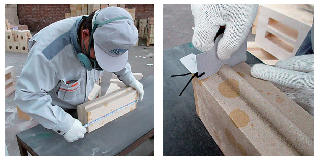
Fig.4 Inspection of silica brick at Sinosteel Refractory Co., Ltd.
