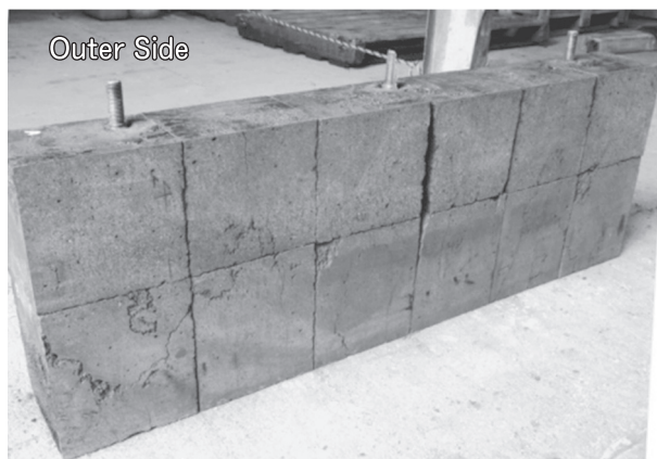
Fig.2 External appearance and cross section of glaze coated door block after 12 years commercial application.
