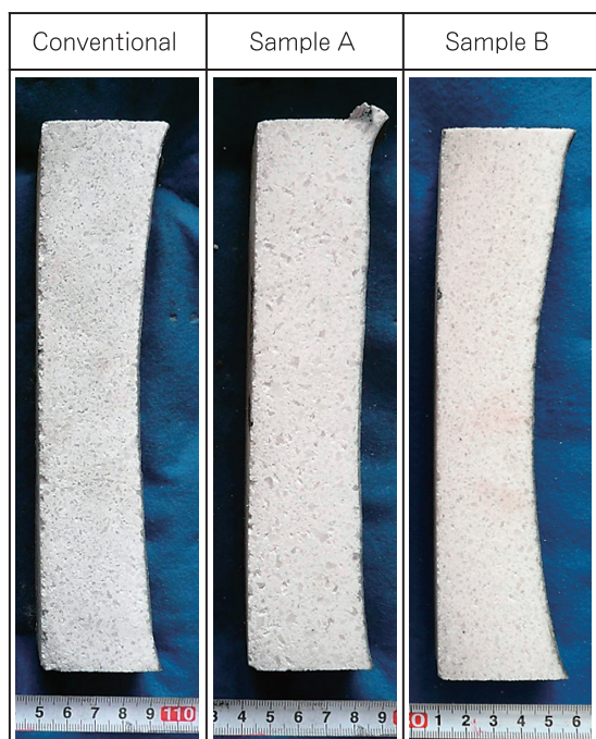
Fig.5 Cross-section of samples after corrosion test.
