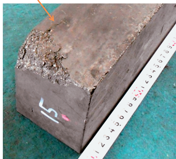
Fig.5 The appearance of the bricks after the test.
