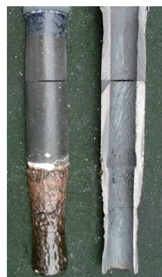
Fig.12 Ladle shroud performance at Caster A and the cut section after use.
