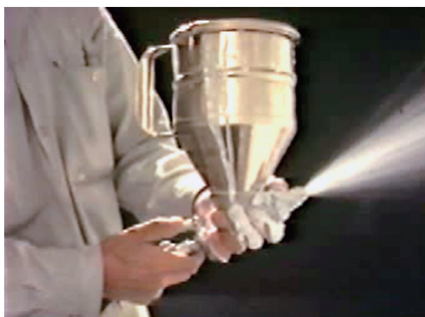
Fig.4 Coating products practice with spray gun.
