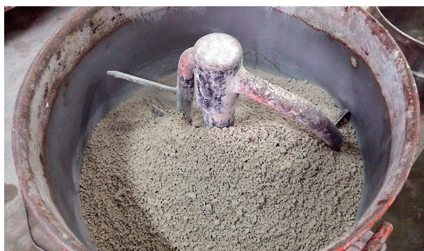
Fig.1 Visual appearance condition of powdery tapping products.
