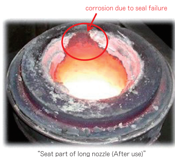
Fig.21 Example of corrosion caused by air suction.
