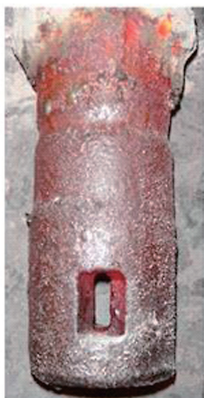
Fig.14 Appearance of “Bend port” SEN after use and comparison of the bleeding defect rate.
