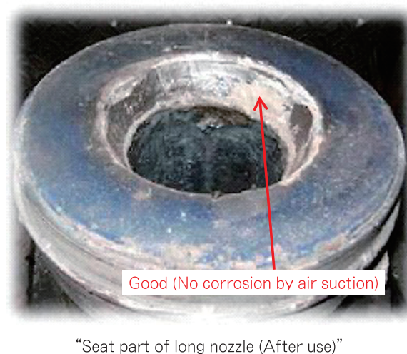
Fig.22 Application of double layer gasket.
