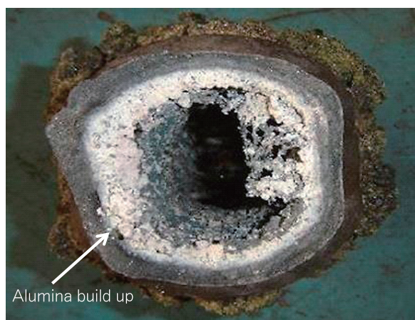
Fig.17 Cross section of SEN used for 6 heats of low carbon steel casting.
