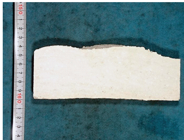
Fig.8 Cross section of gunning sample LX-160G-1.
