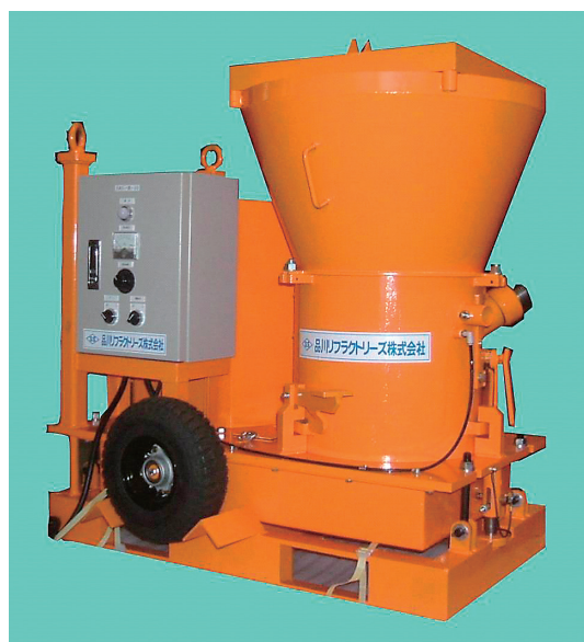
Fig.6 SRG (Shinagawa Refractories Gun).
