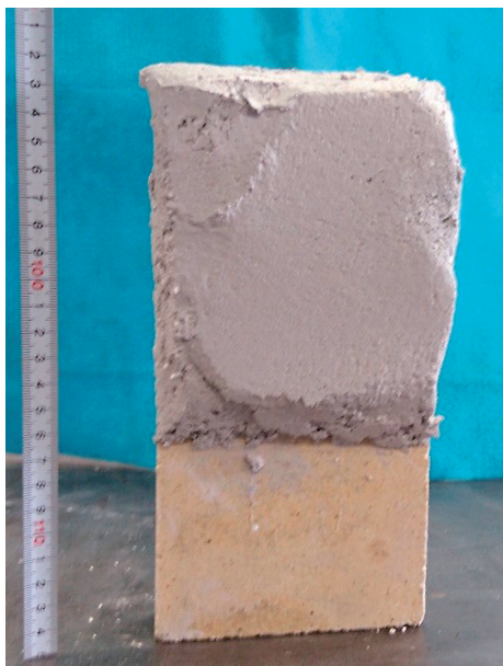
Fig.5 Appearance of troweling material LX-160T-1 application test.
