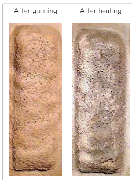
Fig. 4 After heating test.
