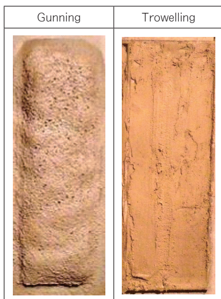
Fig. 1 Appearance of coating material installed by two coating method.
