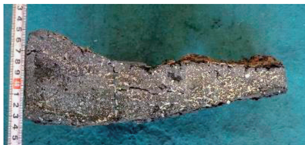
Fig. 12 Cut section of bricks used in impact zone of steel ladle.
