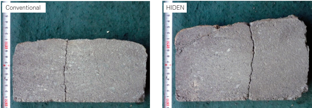
Fig. 11 Cut section of used conventional MgO-C and HIDEN.
