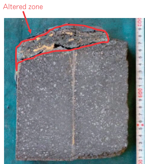
Fig. 15 Cut section of high density \text{Al}_2\text{O}_3\text{-MgO-C} bricks used in impact zone of steel ladle.
