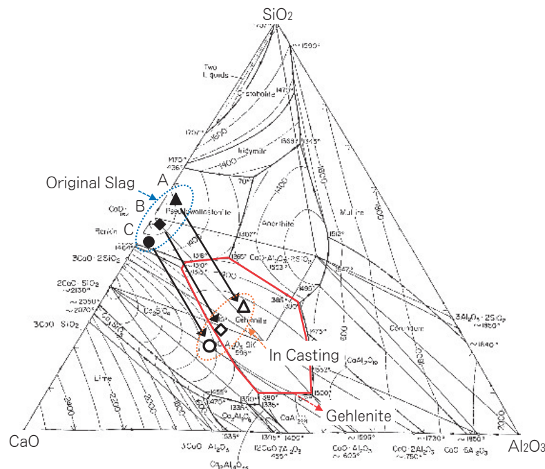
Fig. 3 Change in chemical composition during casting.
