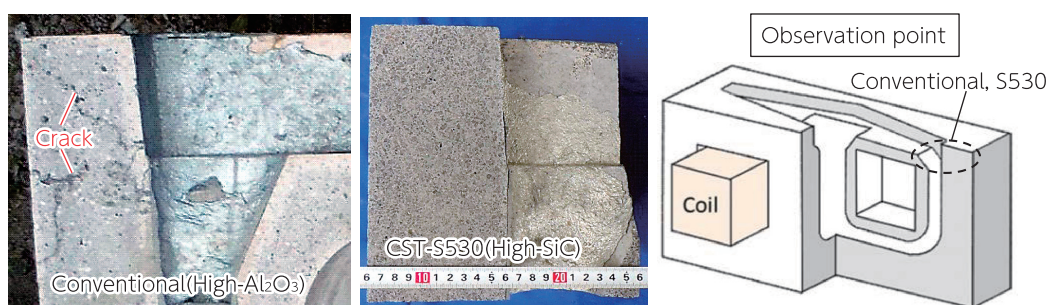
Fig. 7 Cut faces of conventional material and CST-S530 inductor block used in CGL operation for zinc galvanized steel strip.
