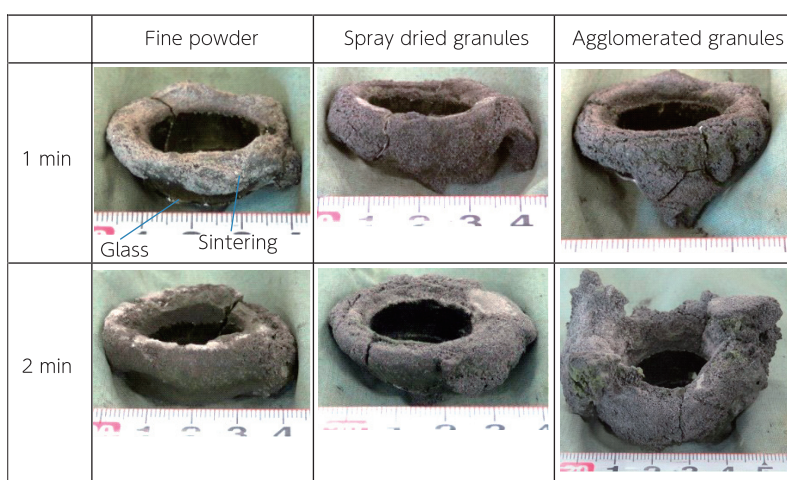
Fig. 6 Appearance of slag roping samples.
