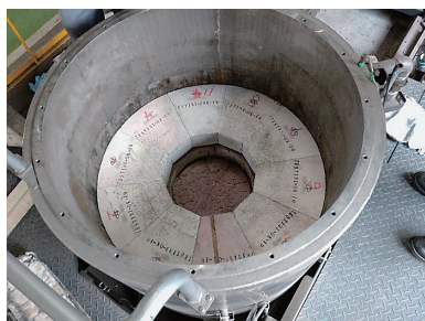
Fig. 3 Appearance of refractory bricks relined in test furnace.
