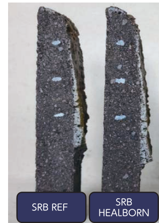
Fig. 8 Cross-section of SRB REF and SRB HEALBORN samples after the corrosion test.
