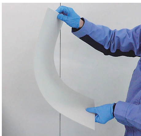
Fig. 3 Appearance LTC-FL (3 × 300 × 600) bent by hand.
