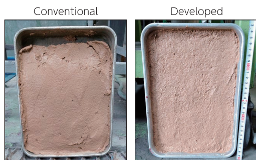
Fig. 5 Test method for evaluating adhesiveness of troweling coating mix.
